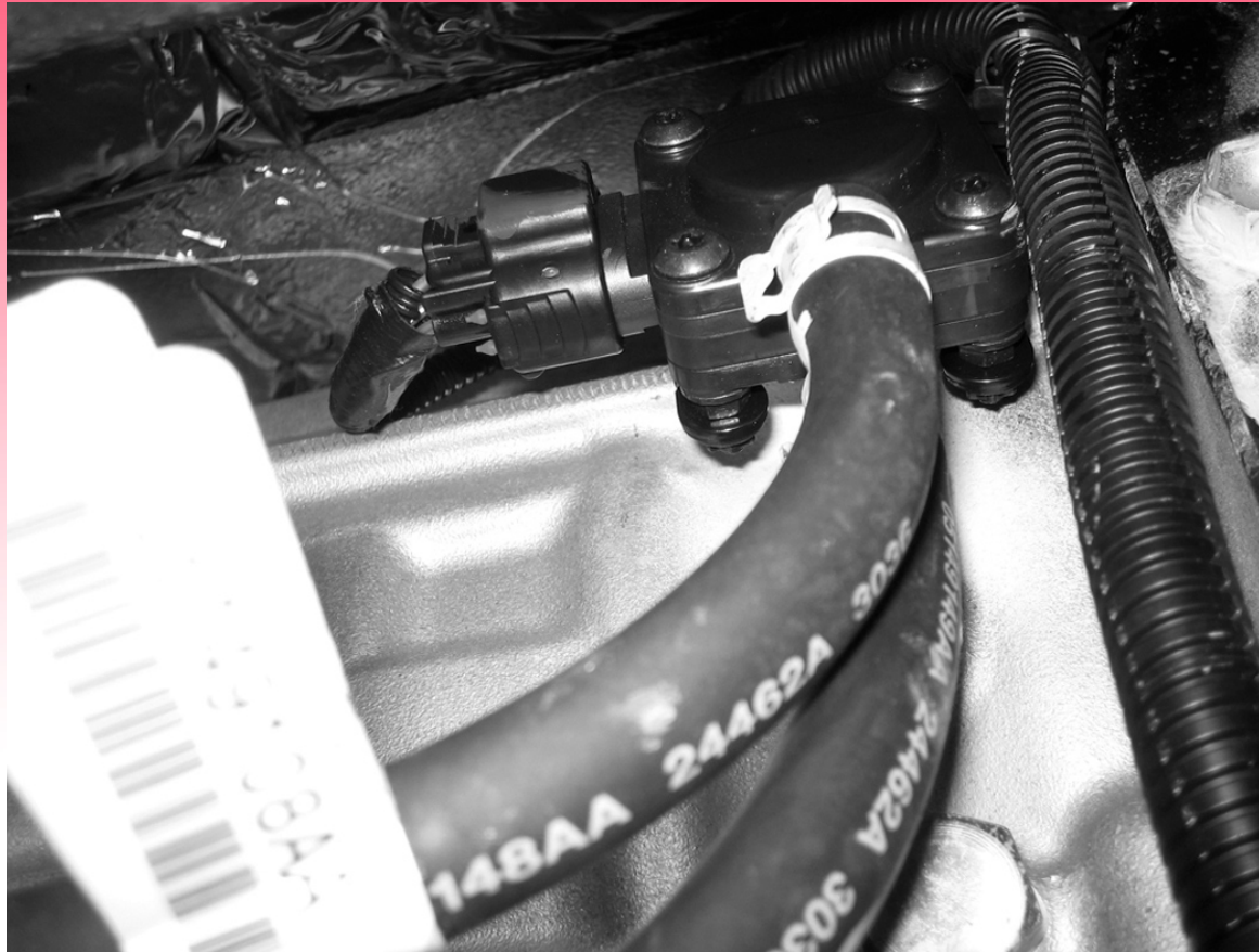
FIGURE 4-19 A differential pressure sensor showing the two hoses from the diesel exhaust particulate filter.
