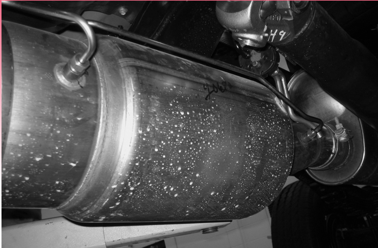
FIGURE 4-18 A diesel exhaust particulate filter on a Cummins 6.7-liter diesel engine.
