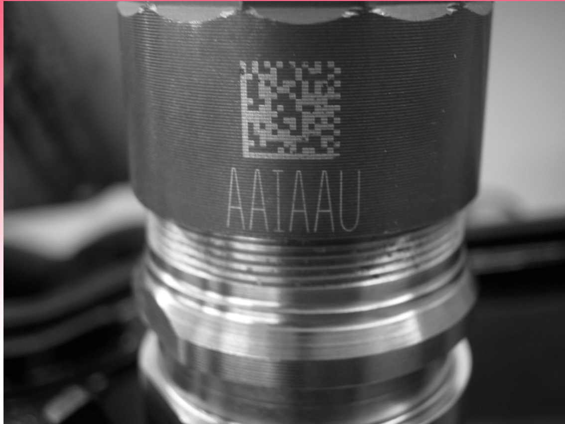
FIGURE 4-23 The letters on the side of this injector on a Cummins 6.7-liter diesel indicate the calibration number for the injector.
