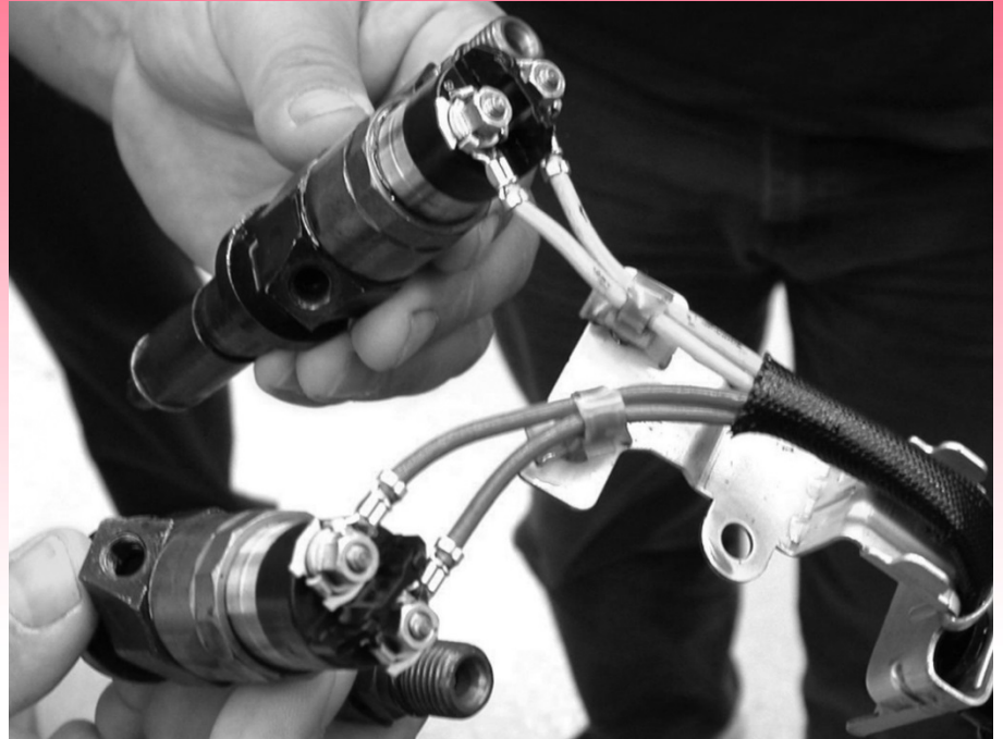
FIGURE 4-12 Typical computer-controlled diesel engine fuel injectors.
